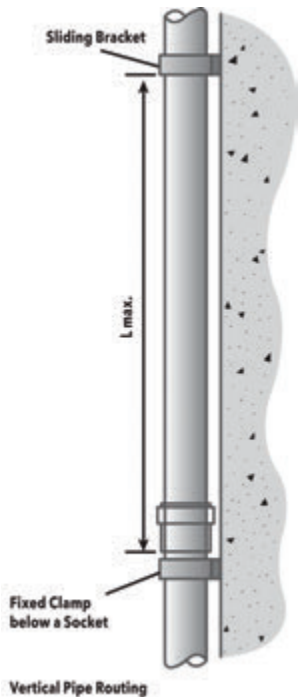
Vertical Pipe Routing
