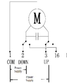
Fig.5: Floating Point Control Wiring 1800/3000/5000N
