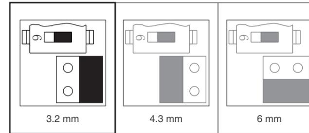
**NOTE: the stroke is factory set at 3.2mm**
