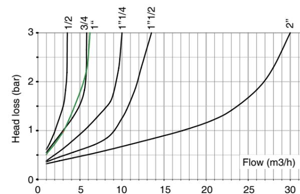
Kv : Flow in m3/h when the outlet pressure become 1 bar lower than its setting at zero.
