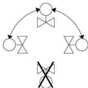
Prohibit downward installation of actuators
