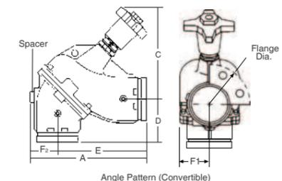
\*Note: Series CSM-91 valves are shipped as straight pattern from factory. To convert to angle pattern refer to instruction sheet shipped with valve.
