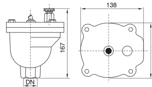
Note: Nominal diameter DN range from 20mm to 32mm
