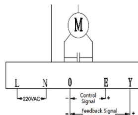
Fig.2: Intelligent Proportional Control Wiring 500/1000/1800/3000/5000N (220VAC)
