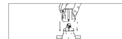
Fig.3 Refit the handwheel so that the V-shaped reference mark lines up with the mark on the valve body. In this position, the handwheel is locked.
