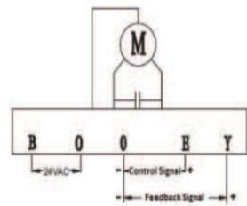
Fig.1: Intelligent Proportional Control Wiring 500/1000/1800/3000/5000N (24VAC)
