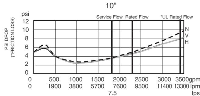
Flow capacity chart identifies valve performance based upon rated water velocity up to 25fps
