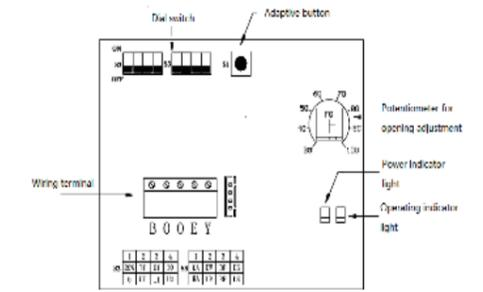
Fig.6: Control Panel - Intelligent Proportional Control 500/1000N (24VAC)
