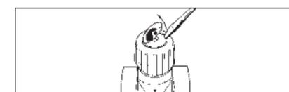
Fig.1 Remove the label with a screwdriver.
