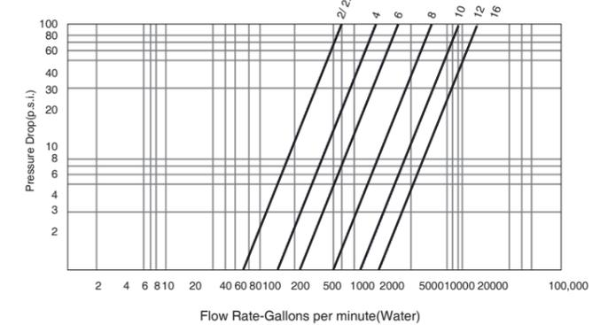
\*NOTE: The Cv Factor of a valve is the flow rate in US GPM at 60° F that will cause a 1 psi drop in pressure.
