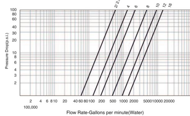
\*NOTE: The Cv Factor of a valve is the flow rate in US GPM at 60° F that will cause a 1 psi drop in pressure.
