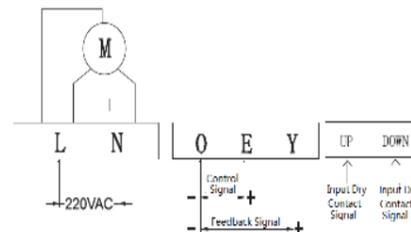
Fig.3: Intelligent Proportional Control Wiring 16000N (220VAC)
