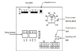
Fig.7: Control Panel - Intelligent Proportional Control 500/1000N (220VAC)
