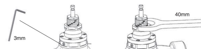
DN40-DN50 Loosen the lock nut before preset, and tighten it
