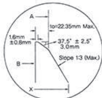
BEVEL FOR WALL THICKNESS(to) 0.88 IN.(22.35mm) OR LESS.
