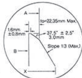
BEVEL FOR WALL THICKNESS (to) 0.88" IN. (22.35mm) OR LESS.
