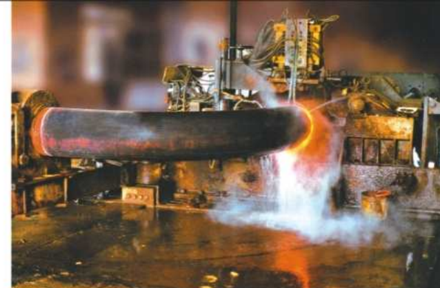
中频弯管机 Intermediate-frequency bend machine
