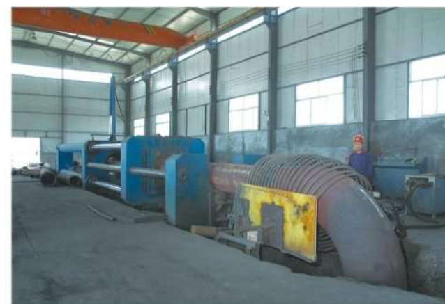
中频推制机 Intermediate-frequency extruding machine
