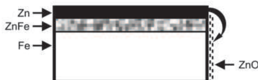
Protection of cut edges with zinc coatings.
