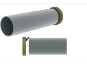
12. Grinding of weld at pipe ends and beveling
