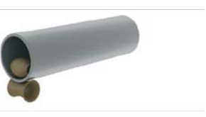
4. Post-bending of the longitudinal plate edges
